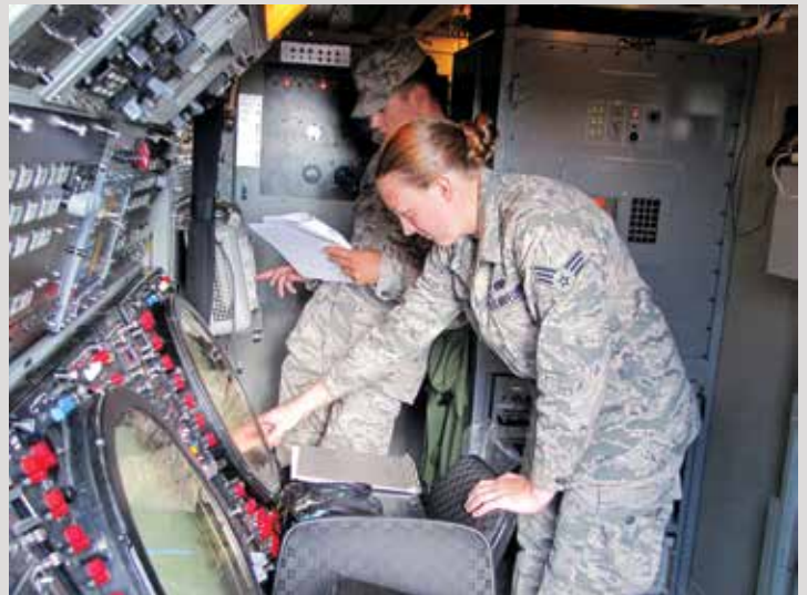
Senior Airman Anastasia Hansen and Airman 1st Class Daxton Arnold prepare an AN/TPS-75, the U.S. Air Force’s primary transportable Aerospace Control and Warning radar, for anti-jamming operations on Aug. 10, 2017, during a field-deployment exercise at Wendover Airfield, Utah.
